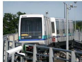
VAL 208 in 2000 with PM in-wheel motors
